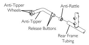
FIGURE 9.2 Installing Anti-Tippers
